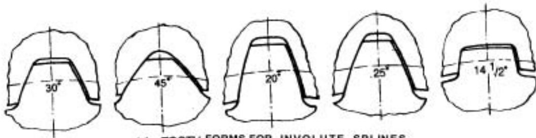
(a) TOOTH FORMS FOR INVOLUTE SPLINES
